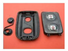
3. Remove old, worn buttons from top part of the shell (buttons are connected with thin piece of plastic)
