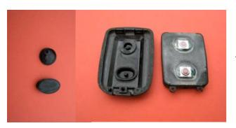
4. Press fit new silicone buttons from outside. Make sure they sit properly and engage with the cover. No gluing is needed.
