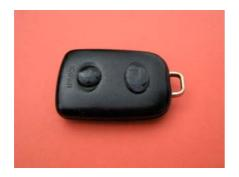
5. Place electronic component over buttons and close whole remote screwing it tightly. Test your remote with the new button fitted in.
